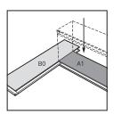
Place an additional panel (B0) on top of panel (A1) to ensure the correct alignment of subsequent panels. This panel will be removed later. Connect the tongue on the short side of panel (A1) to the groove on the long side of panel (B0) by pressing it downwards.
