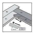
Now, you can install panel (A2) in the same way as panel (B1). Connect the tongue on the long side of panel (A2) to the groove on the long side of panel (A1) at an angle of approximately 20-30°.
