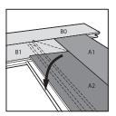
Once the long sides are correctly installed, connect the tongue on the short side of panel (A2) to the groove on the long side of panel (B1) by folding it downwards.
