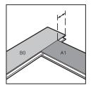
The next step is to connect the next panel (B) to the already installed panel (A1) using an 'angular movement'.
