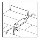
Fit the cover strips along the wall, ensuring they are not fixed directly to the floor. This will allow the floor to expand and contract freely beneath the skirting board. Do not fill expansion joints with silicone or any other substances.
