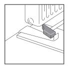
Where it is too difficult to install the panels with a tapping tool (e.g. under radiators), they can be joined together using a tightening tool and hammer.
