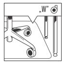
To avoid damage to the floor, secure the legs of furniture and chairs. Use chairs and armchairs with soft 'W' type castors and use appropriate pads. The legs of the furniture must have a large surface area and be fitted with protective caps. The greater the surface area of the furniture legs, the better the weight distribution on the floor and the less risk of damage to the floor.
