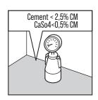
The moisture content of the substrate must comply with national standards for textile floor coverings (carpets):
