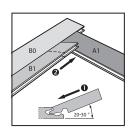
The long sides of the panels should be connected using an 'angular movement'. Insert the tongue of panel (B1) into the groove of panel (B0) at an angle of approximately 20-30°. Slide panel (B1) until the tongue on its short side is positioned directly above the groove of panel (A1).
