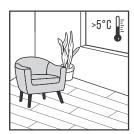
Ensure that the indoor temperature remains above 5°C at all times. The recommended indoor temperature is between 18-30°C. It is also important to maintain the substrate temperature within these limits.
