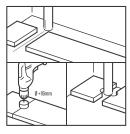
Lay the panels in rows where pipes are present, ensuring that the pipe aligns with the joint line between the panels. Select a drill bit with a diameter that matches the pipe size plus 16 mm. Snap the panels together along the short side, then drill a hole centred on the joint between the two panels. The panels are now ready to be fitted.
