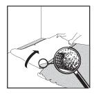
The type, quality, and preparation of the substrate significantly impact the final result of the installation. Keep in mind that uneven ground can cause deformation and gaps in VIN IN products. The substrate must be stable and securely fixed. Additionally, floating floors should not be installed on soft, damaged, or loose subfloors. Overly soft floor coverings, such as carpet, needle-punch carpet, soft vinyl, and previous floating floor coverings, should be removed.
