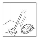
The substrate must be clean, dry, and free from construction debris, sand, mud, and other objects. Any protruding bumps should be removed. Before installation, thoroughly sweep and vacuum the substrate to eliminate all debris.
