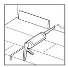
Fit the cover strips along the wall, ensuring they are not fixed directly to the floor. This will allow the floor to expand and contract freely beneath the skirting board. Do not fill expansion joints with silicone or any other substances.
