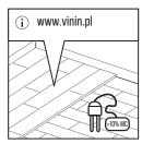
VIN IN panels are suitable for installation on wooden substrates, provided there are no visible signs of mould, dirt, or insect infestation. The moisture content of the wood must not exceed 10%, as the new substrate can trap moisture, potentially causing the wood to rot over time. Additionally, the substrate should be inspected to ensure it is level, and any loose parts must be secured with nails or screws.
