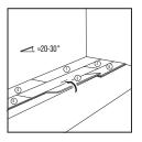
After installing each panel and before moving on to the next, check the connection of all short and long sides. Ensure that no gaps or differences in height are created.
