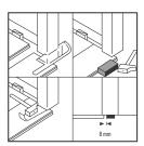
We recommend undercutting the frame profiles at thresholds or doorways. To ensure accurate cutting, turn the panel bottom side up and place it on the floor against the frame. This will allow the cut to be made at the correct height. Then, lay a multi-tool or handsaw flat on the panel and undercut the frame.
