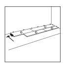
If method A is not possible, e.g. in hard-to-reach areas, method B, which involves hammering the panels, can be used. This eliminates the need to lift them. This method requires the use of a special punch for the UNICLIC snap-in system. The panels should not be joined by single punching. The panels should not be joined with a single punch; instead, tap them gradually to avoid damage. You can position either the short or long side of the panel at an angle first, then tap to join the other side.
