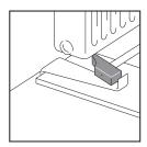
Where it is too difficult to install the panels with a tapping tool (e.g. under radiators), they can be joined together using a tightening tool and hammer.
