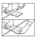
If you need to shorten a panel with a straight cut, position the board with the patterned side facing up and use a vinyl panel cutter. To cut the vinyl panel, draw a straight line to guide the cut. Use a knife to make a secure incision on the surface. It is not necessary to cut all the way through the vinyl panel. Then, break the panel along the cut line using both hands.
