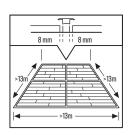
The temperature in the room fluctuates constantly, making it essential for the floor to have the ability to expand and contract. An 8 mm expansion gap should be left on each side of the floor, around pipes, thresholds, and under door frames. Expansion joints can be covered with skirting boards fixed to the walls or with an expansion joint profile. In most cases, an expansion profile is not needed between rooms. However, it should be used if:
